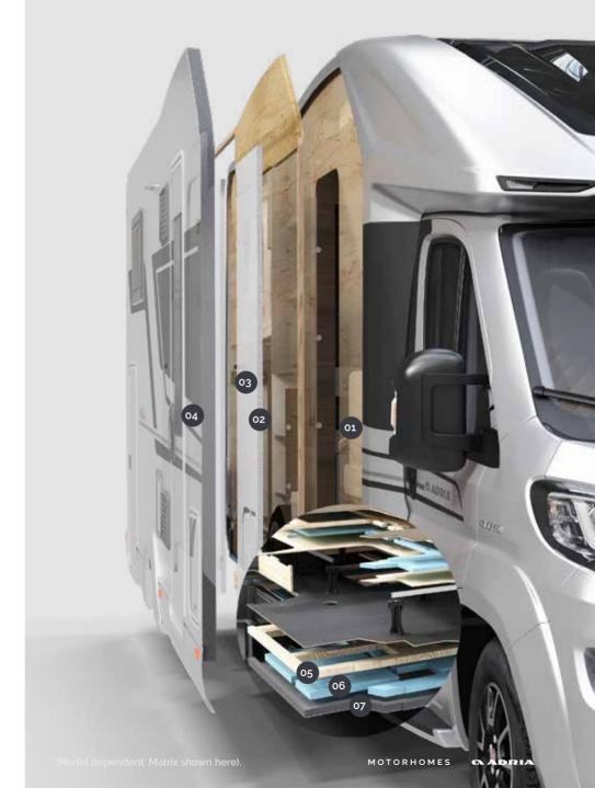
All motorhomes feature a **double floor**, providing a single level floor throughout and 13 cm underfloor space for integrated utilities, insulation and extra storage. Impact resistant **Freshwater tanks** are optimally placed for vehicle balance and handling, formed in a single piece for durable leak-free performance and with easy access via the double floor.
